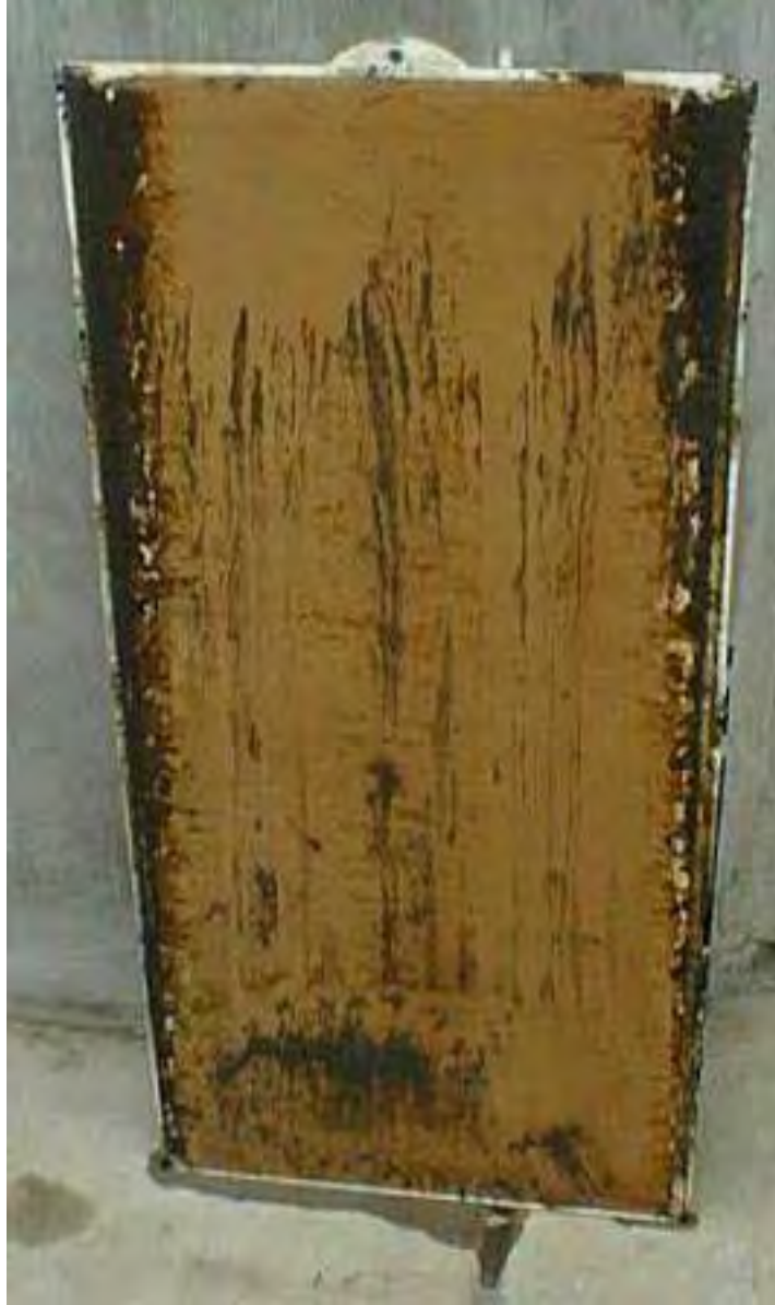
Kubota Type 510 Membrane (after 2 months operation)
