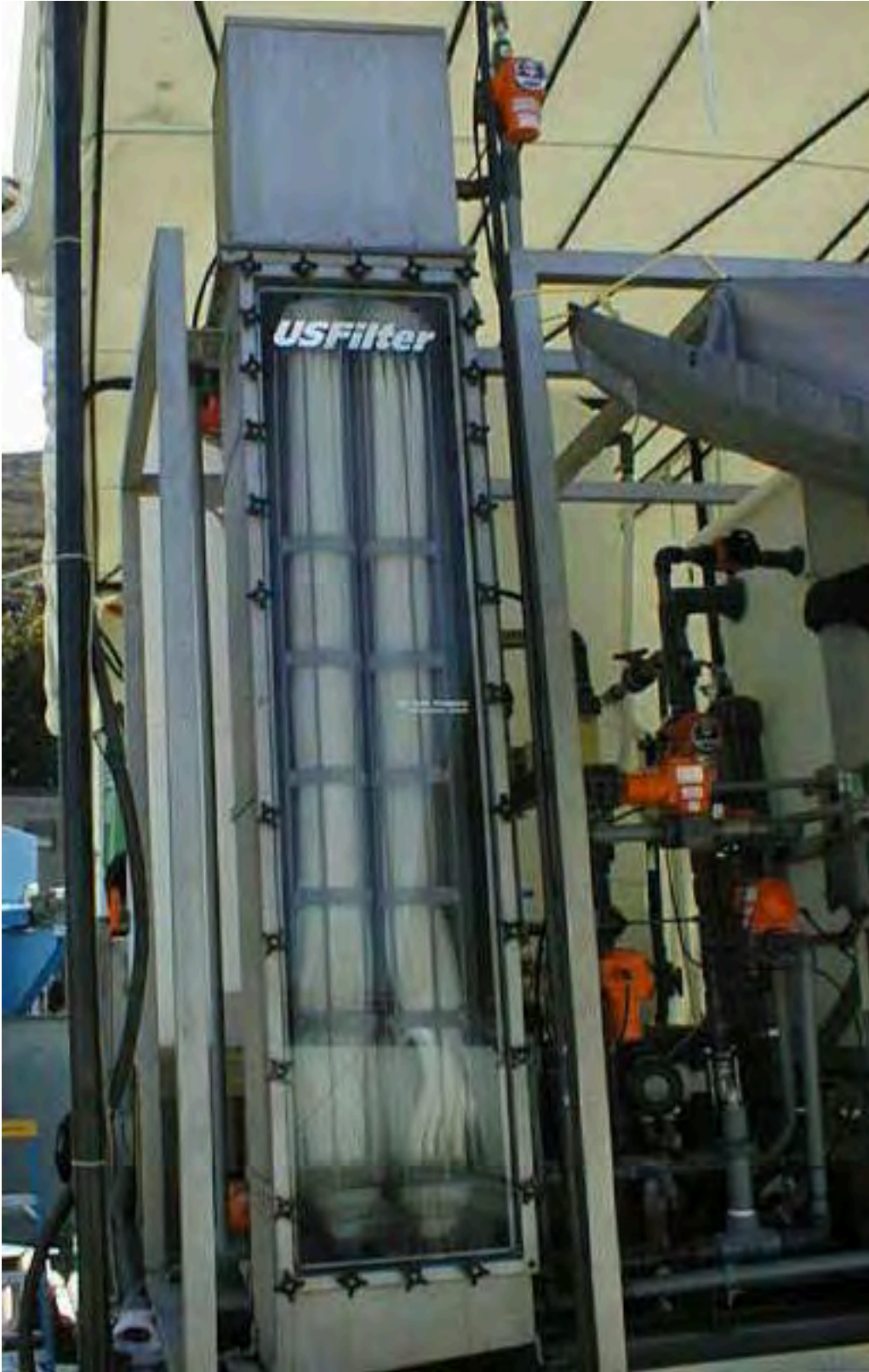
US Filter MBR Pilot Membrane Tank
